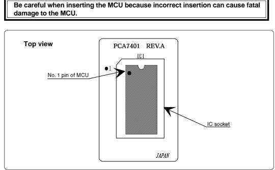
Figure 3.2 Mounting an MCU
